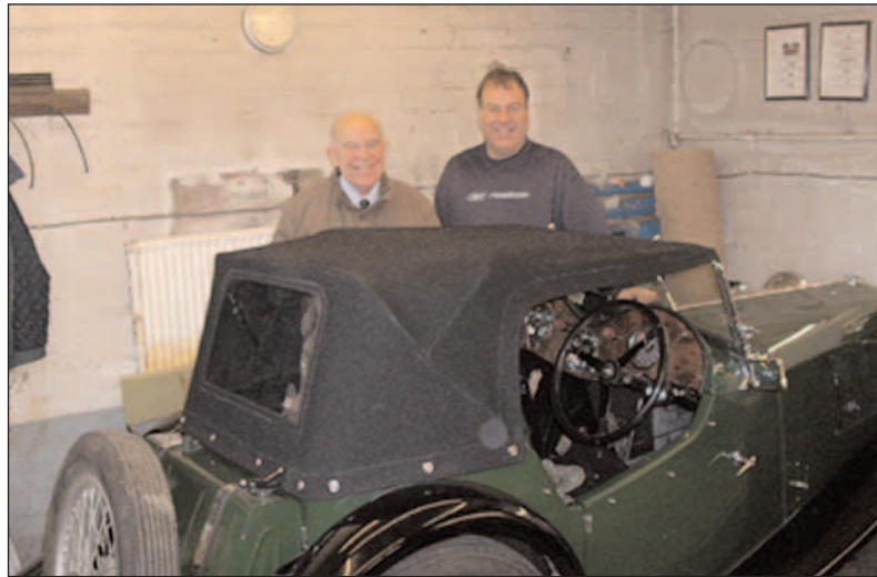
Stan Chilton (left) and Son Phil with the Editorial PA. The hood was designed to allow maximum rear vision and headroom for tall drivers
